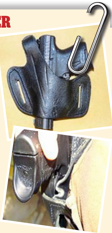
FOLD: Pictures supplied by the whistleblower show how the leather bunches up to potentially catch the gun's trigger
